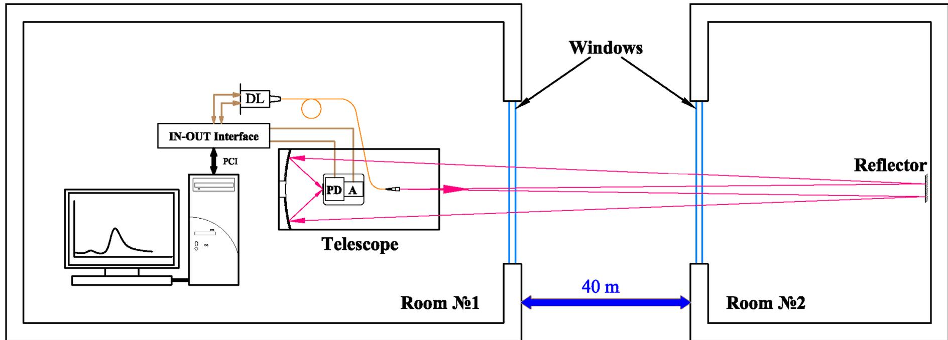
To test the scenario of human presence remote detection  $\text{CO}_2$  channel of the instrument developed was used. The instrument was installed in room №1. Collimated laser beam was directed through room windows to windows of room under control located in other building. Distance between buildings was 40 m. Scattered light was detected by receiving optics and focused on PD.
