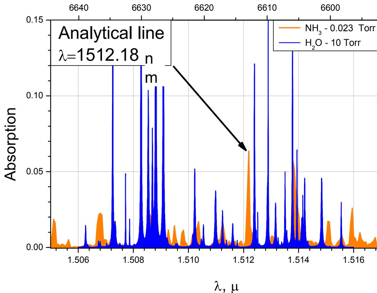
Choice of analytical line for ammonia detection taking into account interference with water absorption.
