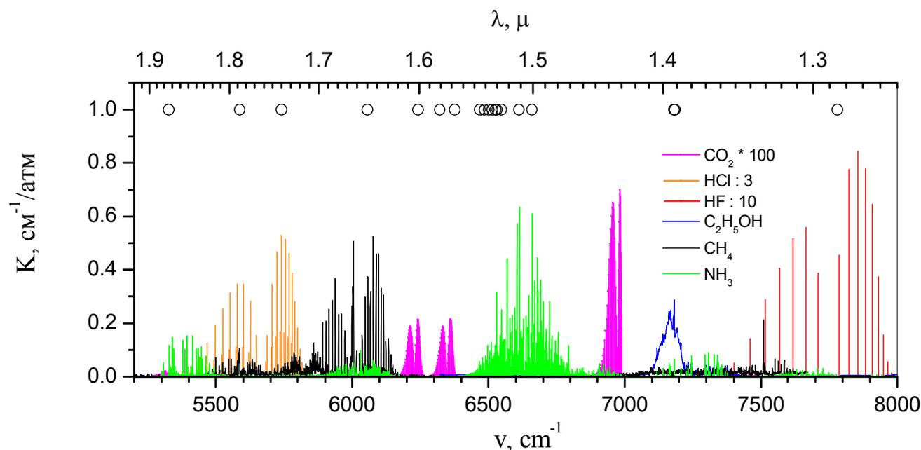
Absorption spectra of several molecules in near IR spectral range
