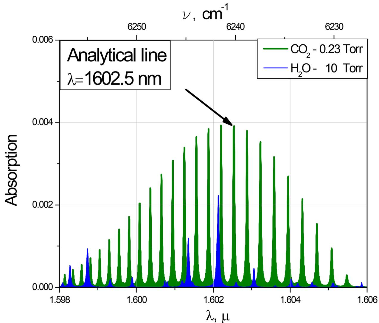
Choice of analytical line for CO<sub>2</sub> detection taking into account interference with water absorption.
