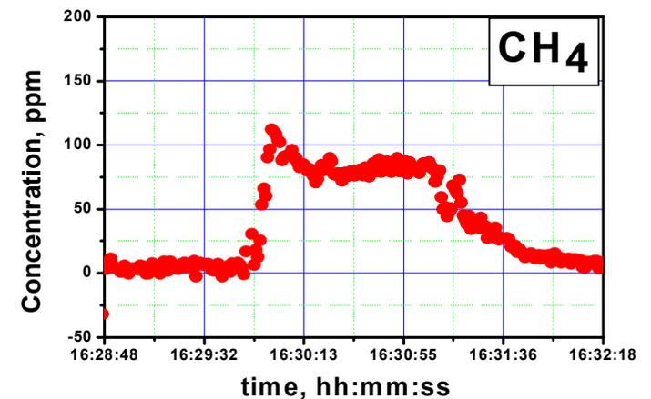
Remote detection of ammonia and methane when sample gases were injected in vehicle located at 100 m from instrument. Fiber amplifiers were used to increase receiving signal. **Simultaneous detection at the same time of all molecules under consideration is signature of human presence.**
