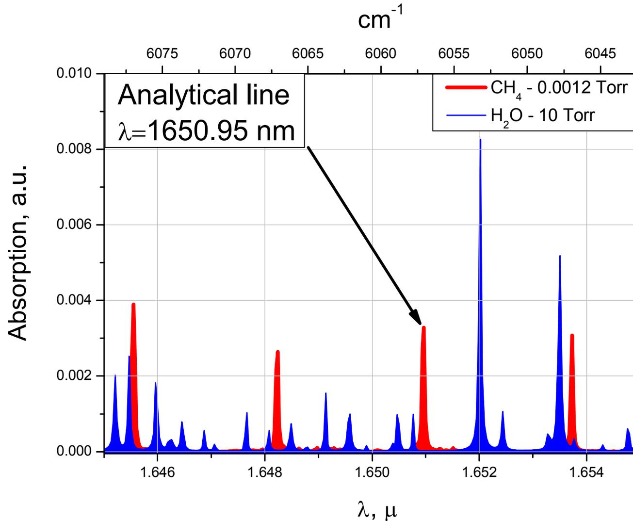
Choice of analytical line for methane detection taking into account interference with water absorption.
